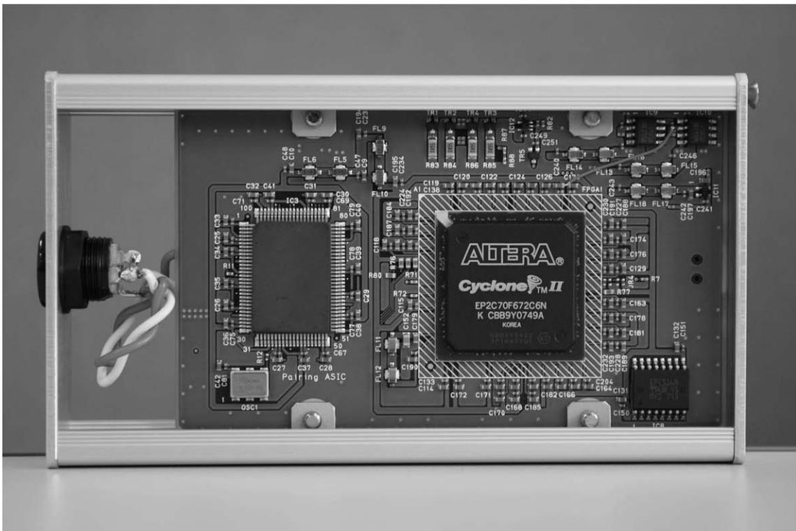
Fig. 6. Evaluation board for the PairingLite chip.
